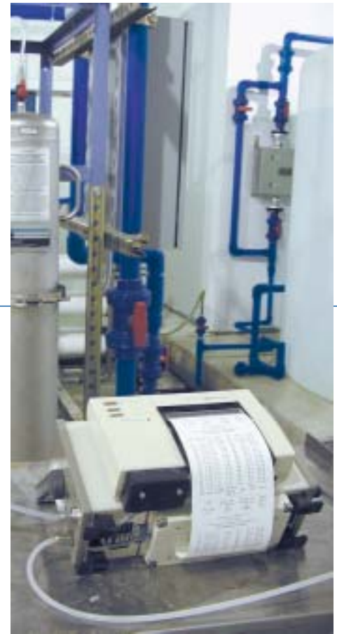
On-line TOC is measured continuously on the return side of the loop.
