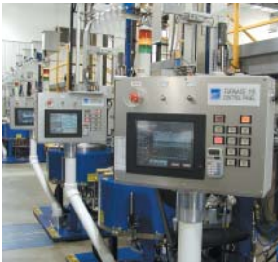
Silicon growth furnace controls at Ebara Solar are highly automated.
